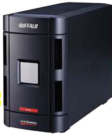
▲ LinkStation Pro Duo uses RAID technology to either improve drive performance or reduce the risk of data loss
