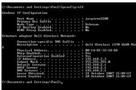
▲ Your router can accept connections from a preferred list of MAC addresses to prevent outsiders tapping in
