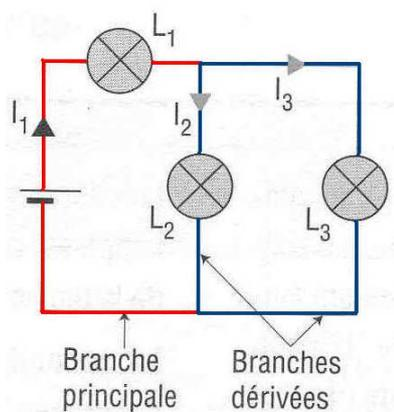
$$I_1 = 280 \text{ mA}, I_2 = I_3 = 280 : 2 = 140 \text{ mA}$$
